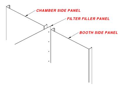
Following the exploded view drawings, continue alternately assembling wall panels and roof panels to each other until you reach the front end of the booth. Finish off the roof section by attaching the fire curtain if needed. If booth has doors, no fire curtain is needed.
