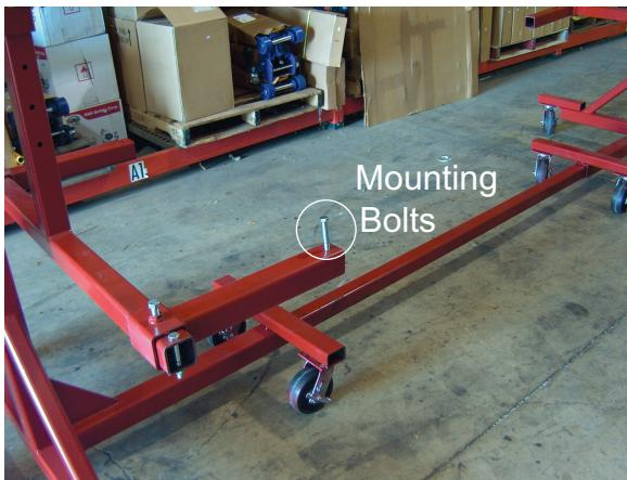
Lift vehicle and bolt vehicle frame to Frame Supports using supplied mounting bolts.
