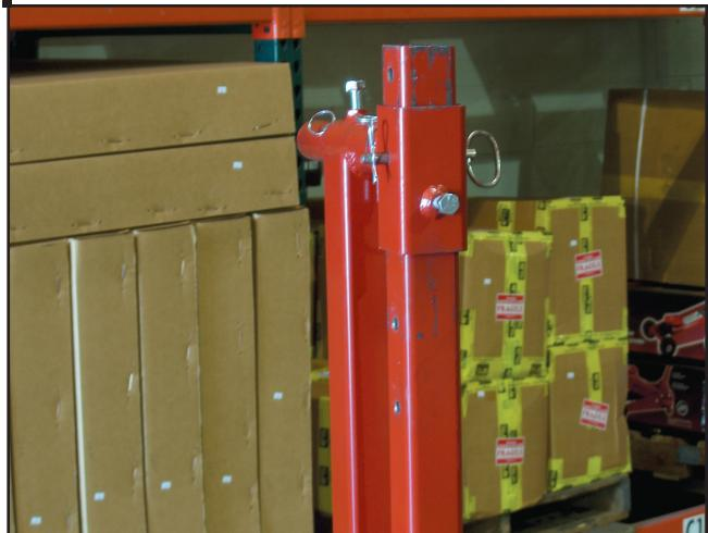
Insert Bracket Arm Support into Bracket Swivel. Adjust to desired height and lock into place with locking pin.
