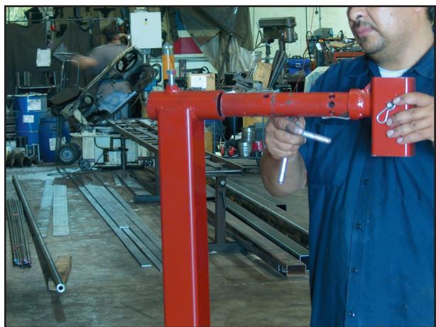
Insert Bracket Swivel into Base Mount. Applying a light layer of grease before inserting will allow for easier rotating of vehicle.
