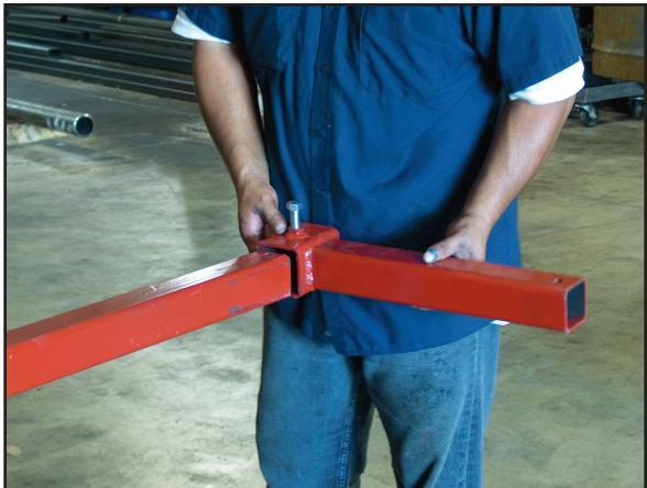
Insert Bracket Arm into Bracket Arm Support. Adjust to desired width to align with mounting holes on vehicle frame and tighten locking bolt securely.
