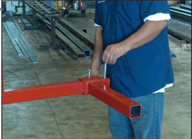
Insert safety pin at end of Bracket Arm Support. Repeat steps 4 and 5 for installing Bracket Arm on other end of Bracket Arm Support
