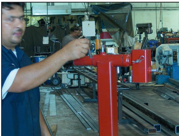
Insert locking pin to hold swivel in place
