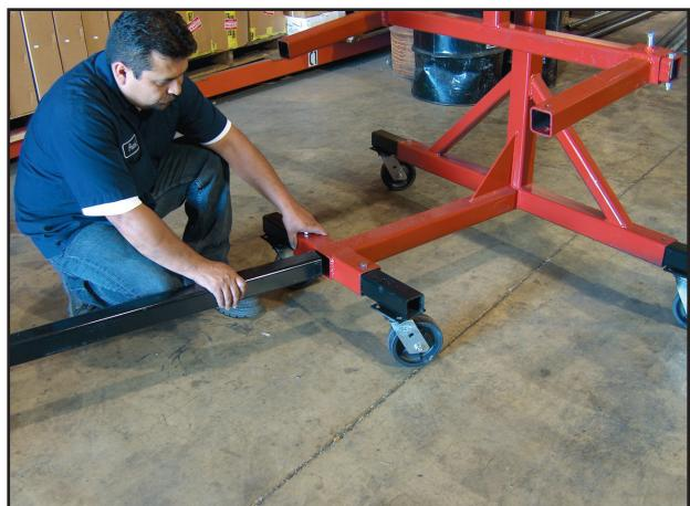
Insert Beam into Frame Supports.
