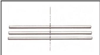
If all bars appear to be parallel and all pointers appear from sighting along the center line to be in a common fore and aft vertical plane, it can be assumed that the frame is in alignment. Any deviation indicates the frame is in need of correction.
