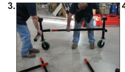
Connect it to the short arm of another Corner Support. The Frame Brackets on top of the Corner Brackets should be facing the same way.
