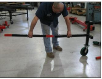
Insert Extension Arms into Corner Dolly Supports. Start by by installing the Extension Arm into the long arm of one of the Corner Supports.
