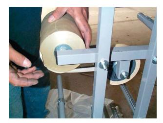
Pull tape and attach to paper roll. Make sure the tape overlaps the paper roll to have an exposed edge of tape to stick to surface to be painted.
