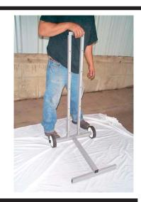
Attach long paper holder to vertical bracket in the bottom holes with bolts.
