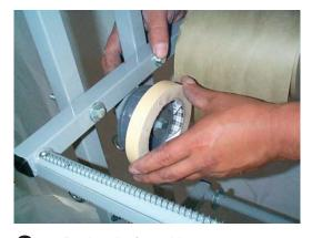
Push roll of masking tape onto tape holder. Make sure it is snug.
