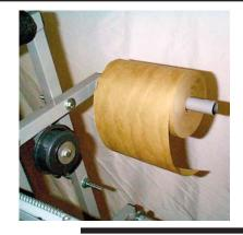
Slide paper roll onto paper bar as far as it will go. Add washer and paper lock. Tighten paper lock to hold paper roll in place.
