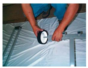
Attach wheels to bottom support base. Push on wheel anchor cap.
