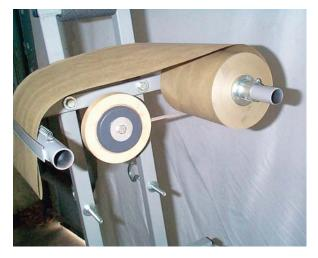
Insert paper with tape into paper cutting guide. Make sure you go over the spring. Do not put paper under spring or tape will stick to bar.
