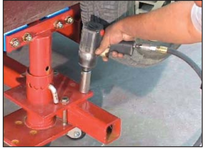
Tighten Pinchweld Brackets securely to Bracket Arms.
