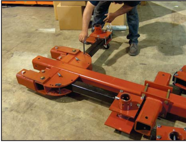
Remove locking pin and swing out Clamp Arm. Install locking pin to lock Clamp Arm into place
