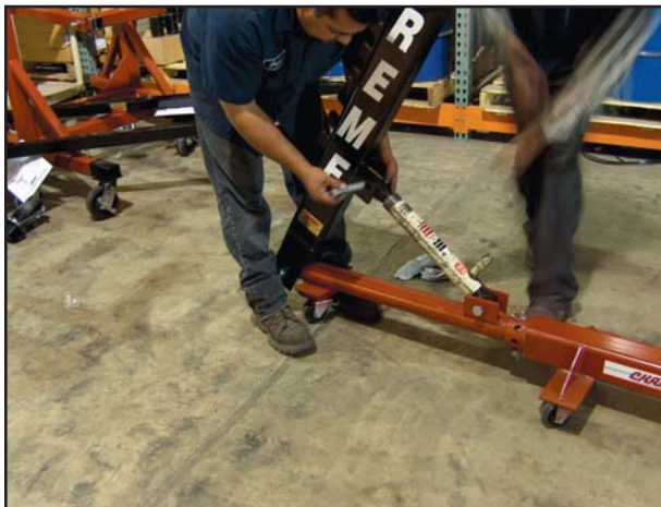
Remove Ram Coupler from Pulling Tower and screw onto Hydraulic Ram. Attach Ram Coupler to Pulling Tower using supplied bolt. Repeat steps for second Pulling Tower.
