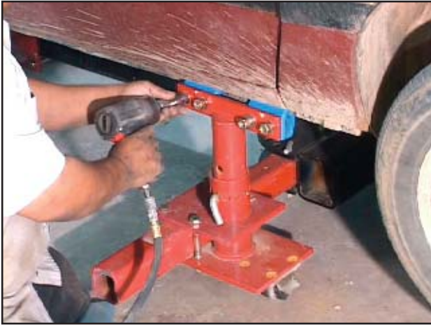
Tighten Pinchweld Clamps securely onto vehicle pinchwelds.
