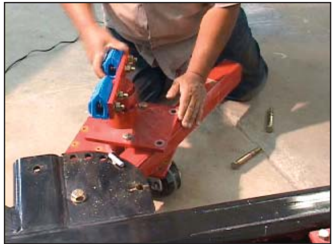
Remove Pinchweld Clamp Brackets.
