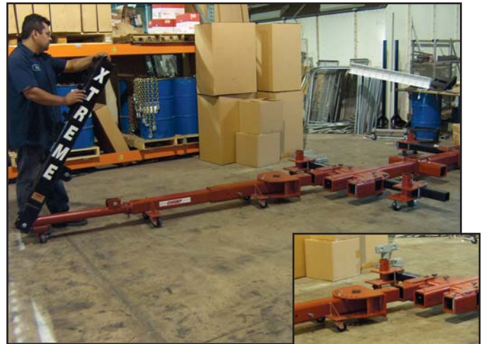
Insert assembled Pulling Tower into each of the Six tower inserts. Lock into place with Locking Pin.
