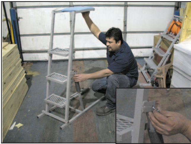
Lift support arm. Remove locking pin from Pad & Step Assembly. Position support arm into Pad & Step Assembly and insert locking pin. This will lock support arm into place. Repeat for other side.
