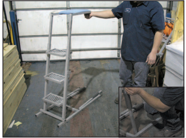
To lock into working position: Lift pad & step assembly
