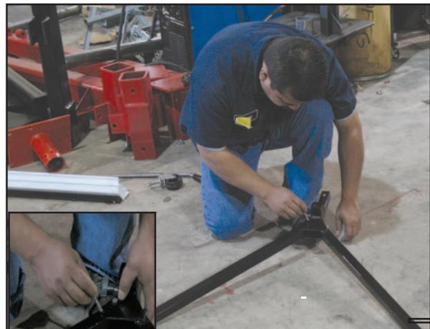
Insert the screws into each hole of the base.
