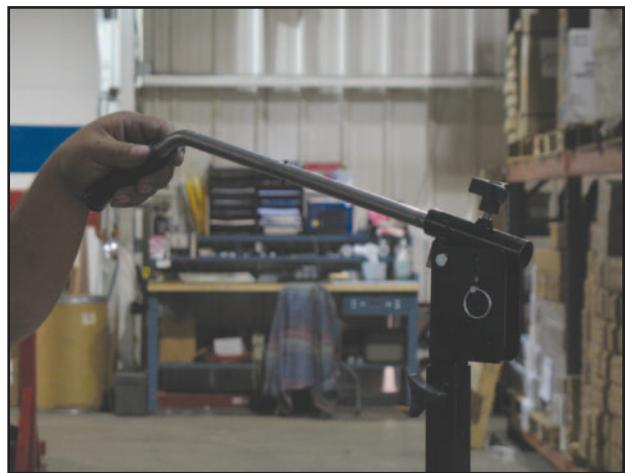
Insert the light handle into the light holder. The handle should go all the way through the holder until you see a hole for a screw come out the other end. Tighten the knob to keep the handle in place.
