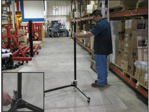
Insert the 47" metal tube into the base and tighten the knob to keep the tube steady.
