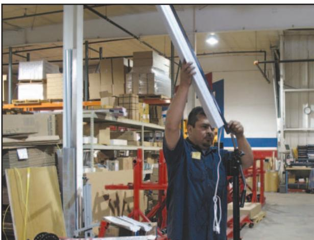
Take out the screw on the light. Insert the light on the end of the handle. Align the hole on the handle with the one on the light.
