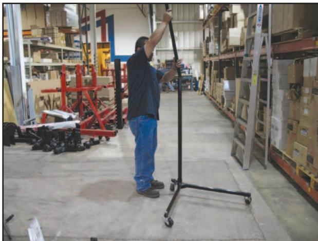
Insert the 53" inner tube into the 47" tube.
