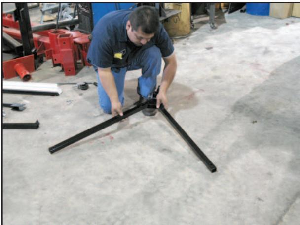
Unfasten the two screws in the base and insert the leg. The holes will align.
