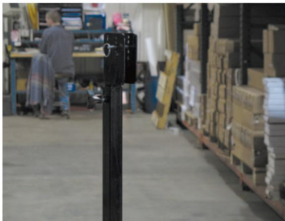
The height of the inner tube can be adjusted by placing it at the desired height and tightening the knob.
