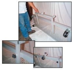
Attach support arm extension bracket to base and tighten with tension knobs. Attach small caster to bottom of support arm extension bracket
