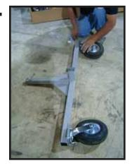
Attach large caster wheels to both Support Bases with included nuts bolts & washers
