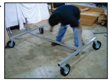
You can adjust the width between the Support Bases by sliding the Support Crossmember in & out of the Bases. Lock into place with the Lock Bolts.
