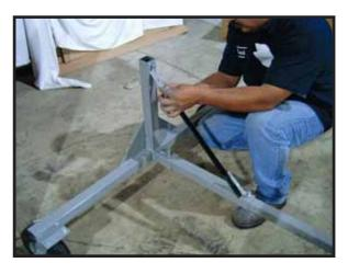
**5.** Attach Base Support Bracket to Vertical Base Support & Support Crossmember. Repeat for both sides.
