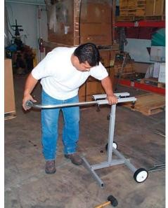
• Insert bumper support arms into arm holders. Screw in tension knobs
