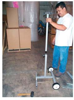
Insert support stand extension into support stand. Screw in tension knob on support stand. This allows for height adjustment. 4.
