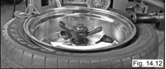
1. Move the Upper Bead Breaker Roller to its highest position.
