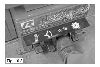
5. Release the inflation pedal. Verify that both beads are completely sealed to the wheel. Repeat these steps if beads have not sealed. It may be necessary to wait a few seconds for the air storage tank to recover before attempting again. If tire and wheel are properly lubricated and operator
