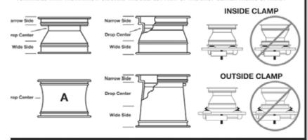
(ARNING: The wheel illustrated above in diagram "A" has little or no prominent drop center. These are not DOT pproved wheel configurations. The tire or wheel - or both - can be damaged during mounting procedures causing the re to explode under pressure, resulting in serious injury or death. If you attempt to mount/demount this type of wheel, se extreme caution.
