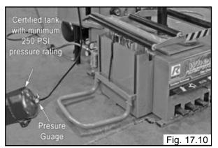
3. Depress inflation pedal to start air flow through the hose and into the tank. Maintain a steady pressure for constant flow.
