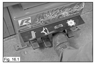
Tire Inflation – This is the activated position. With the inflation hose attached to the tire valve and the pedal depressed, line pressure is allowed to flow through the valve and into the tire for inflation. Tire pressure is indicated on the gauge in this position. (See Fig. 16.2)
