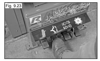
2. Each time the Tool Head Control Pedal is depressed the Tool Head will rotate. (See Fig. 9.24 & 9.25)
