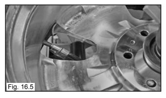
Hold tire up against upper edge of the wheel. Be sure tires top bead is over the bottom of the valve stem. (See Fig. 16.6)
