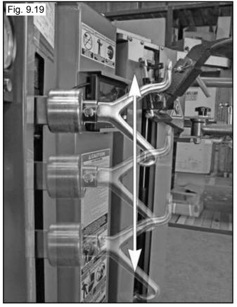
1. Using the Joystick on the Control Pod to Retract and Extend the Tool Head Assembly In or Out. (See Fig. 9.20)
