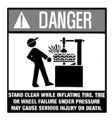
1. Once tire pressure is indicated on the air gauge (inflation pedal depressed, continue to inject air into the tire in short intervals. Check the pressure frequently. Stand back during bead seat. Keep hands, arms, and entire body away from tire during this procedure. Tire beads should move outward and "pop" into their bead seat position as pressure inside the tire increases. If this does not happen, a problem exists. Investigate carefully. (See Fig. 16.10)
