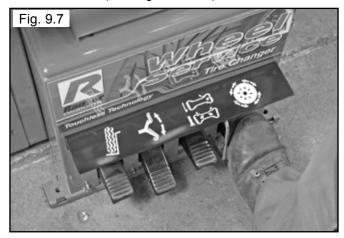
3. Pull **UP** on the Turntable Rotation Pedal to rotate counter clockwise. (See Fig. 9.8 & 9.9)
