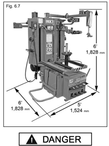
These measurements are the tire changer's working range. Persons other than specially trained and authorized operators are expressly forbidden to enter this area. Choose a safe location that is in compliance with current work place safety regulations.
