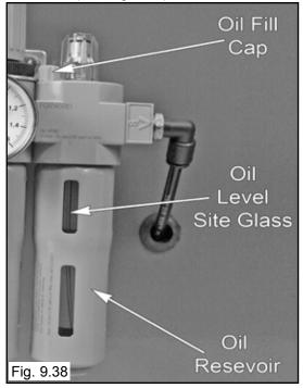
4. The Oiler is adjusted by turning the Small Screw located on top of the Oil View Glass. (See Fig. 9.39)
