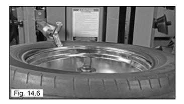
2. Lower The Upper Bead Breaker Roller and if needed, position the Assist Arm Roller to press the Upper Bead into the drop center of the Rim. (See Fig. 14.7)
