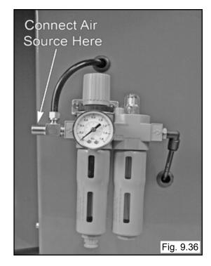
2. The incoming pressure to the Tire Change is adjusted using the Pressure adjustment Knob. Read the incoming pressure on the Incoming Pressure Gauge. (See Fig. 9.37)
