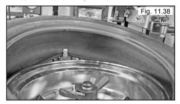
9. Keep the Lower Bead in the Drop center of the Rim.
