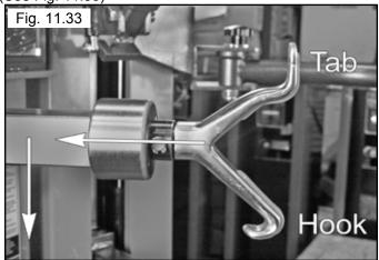
4. Position the Drop Center Tool as shown to bring the lower Bead up onto the Tire's Drop Center. (See Fig. 11.34)
