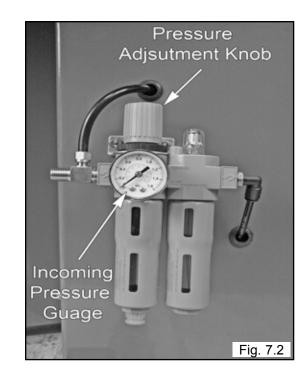
3. Drain water, fill oil and adjust the flow of oil as shown on page 27.
