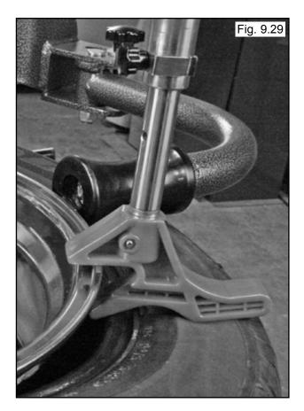
2. Lifting or supporting the under side of the tire to help Center the Lower Bead into the Drop Center of the Rim when Mounting. (See Fig. 9.30)
