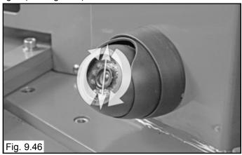
4. Adjust the Camera so as to see the lower edge of the Rim where the Tool Head Tab nears the Rim. (See Fig. 9.47 & 9.48)
