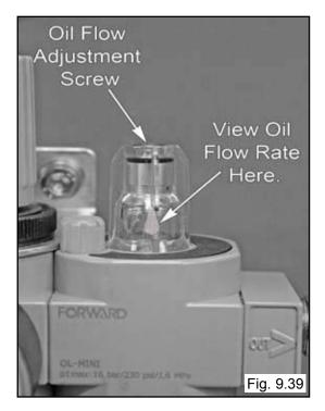
5. Adjust the oil flow so that two to three drops are visible through the Oil Flow Site Glass when operating the Wheel Lift.
