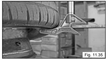
6. Push the Target Lock<sup>™</sup> button and Hold, the Tool Head Tab will extend to the preset position 1/4" from the rims edge.
