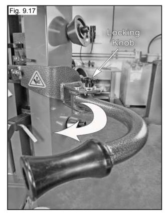
5. Use the Locking Knob to lock the Bead Roller Arm in position after placement.
