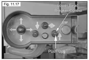
22. Pulse the Upper Bead Breaker switch down in small increments and the Lower Bead Breaker control up as the tire rotates to complete breaking both the Upper and Lower Beads. (See Fig. 11.18 - 11.19)
