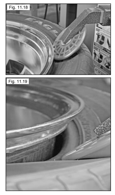
23. Use the Center Post Control and bring the Turntable Assembly back so the rim edge is 1/4" away from the Bead Breaker Rollers.
