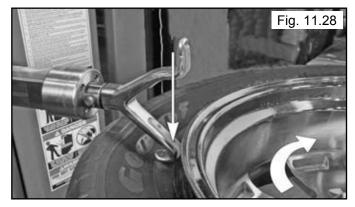
31. Continue moving Tool Head Hook down and in until the Tire Bead pops under the hook. (See Fig. 11.29)
