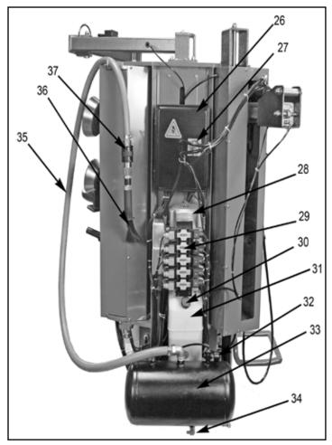
(26) Power Center — Houses relays fuses and wiring components.
