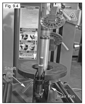
3. Align the holes and replace the Shaft pin and Hair Pin.
