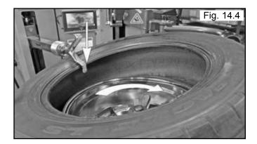
4. If necessary, for some stiff sidewall tires, use the Upper Bead Breaker Roller to help push the down on the tire, to Push bead below rim lip. (See Fig. 14.5)
