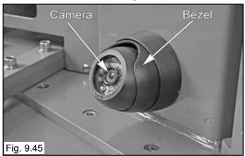
3. The Camera angle of view can be adjusted by rotating the Camera mounting bezel up, down, left and right. (See Fig. 9.46)
