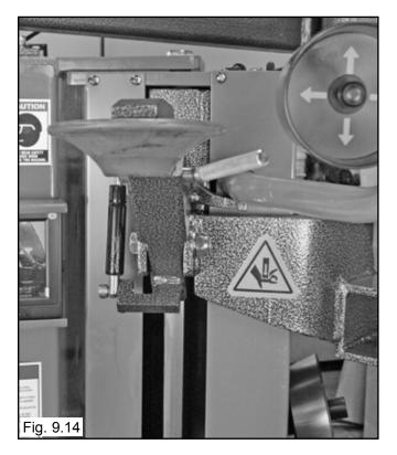
4. To flip down the Upper Bead Breaker Roller without rasing the Roller to top most position Press on the Release Lever.
