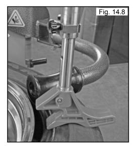
4. Lower the Drop Center Tool to Push the Upper Bead below the Rim's Drop Center. (See Fig. 14.9)
