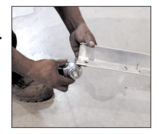
• Attach wheels to base using the 1/2" lock washers and 1/2" lock nuts.
