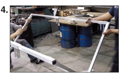
• Attach the 60" top bars to the cross bars. Make sure that the sliders are pointing down towards floor like in the picture above
