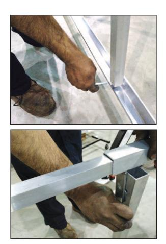
• Use the 5/16" bolts, 5/16" lock nuts and washers to attach the vertical tubing to the base and the sliders.
