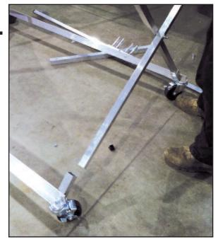
• Lock wheels to keep base from moving. Insert the 46-1/2" cross bars into the angled square tubing area on the base.
