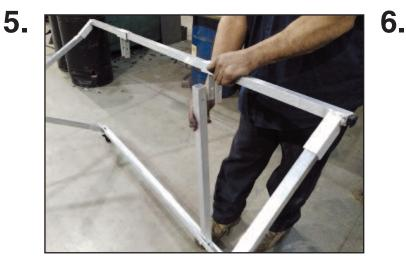
• Attach the 4 - 29" square tubing pieces. Each piece connects to the base and to the sliders on the top bar.
