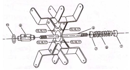
**4:** Align larger center holes and insert the Axle (#4). Install four Long Bolts (#15), four Small Locknuts (#16) and eight Small Washers (#17) into four inside holes. Tighten all bolts and locknuts securely.
