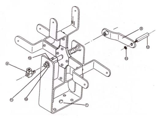
**6:** Install the Large Washer (#10) on the Hexagon Adapter. Insert it into the larger hole on the Base (#1) and install another Large Washer (#10) and Retaining Ring (#11). On the other side face of the Base (#1), clockwise rotate the Handle Shaft (#5) and hand tighten it securely.
