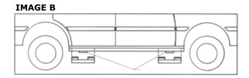
Locate each adapter so it straddles each lifting tab equally (Image B). This will provide a vertical flange long enough for a double-jaw rocker clamp on each torque box area.
