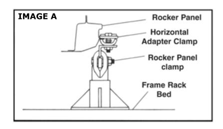
The cutaway view (Image A) shows how the Champ Horizontal Pinchweld Adapters fasten to any standard vertical rocker clamp on all holding systems. The 1990 Honda Accord has a horizontal pinchweld instead of the normal vertical pinchweld found on the rocker panels of most vehicles. There are 4 small lifting tabs which appear as vertical pinchwelds. These small tabs are externally mounted pieces of sheet metal which are intended as jacking points for the car.
