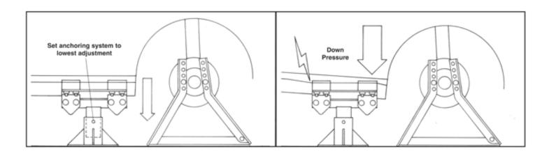
Set anchoring system to lowest setting to keep the center of gravity as low as possible. Use of wheel supports will determine correct height to set anchoring system.
