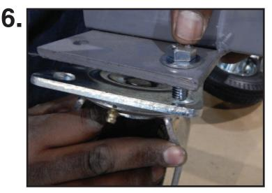
Attach the (4) casters to the (2) base support beams. Slide the bolt through the washer and then through the base support beam and caster. Fasten with the lock washer and nut. Next, install the (12) end caps
