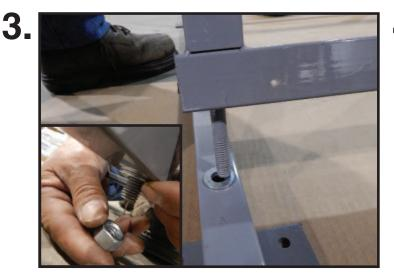
Insert the pre-attached bolts on the side rails (B) into the pre-drilled holes on the base support beams (A). Fasten with bolt.
