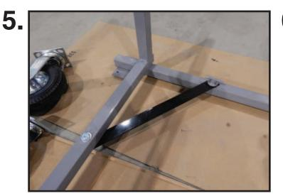
The above pictures shows how the support bar should look once attached to the side rail.
