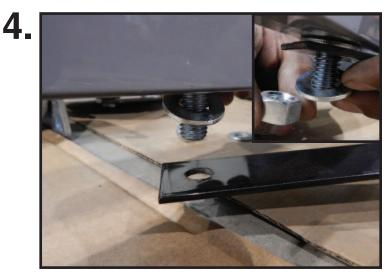
Attach the support bar to the bottom of the side rail (B) and fasten with bolt. (Make sure to place a washer on top of and below the support bar. See the above pictures)
