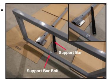
The next step is to attach the side rails (B) to the base support beams (A). When laying out the side rails, make sure to have the side rail with the support bar bolt, next to the base support beam that has the support bar, like the above picture.
