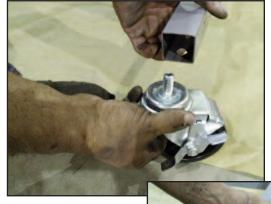
• Attach wheels to base using the 1/2" lock washers and 1/2" lock nuts.
