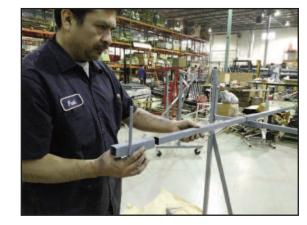
• Attach the the sliding hood adjusters to the 65" square tubing. They slide on and can be adjusted when attaching a hood to the hood rotisserie.
