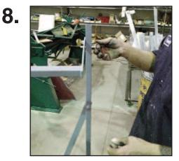
• Insert pin through vertical square tubing and the rotating bar.
