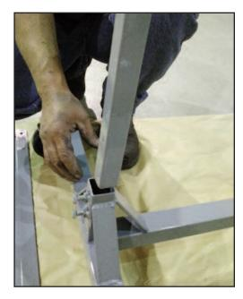
• Insert 47" tubing to both sides of the base.
