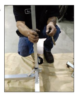
• Insert square tubing to base using the two 3/8" bolts.
