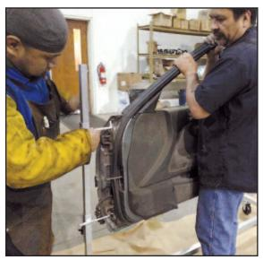
• To take your door off your car, remove the pin that secures the door to the car. Line the slider hooks on the Champ Aluminum Door Stand with the hinge on the door.
