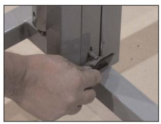
Re-install black plate onto bottom of Panel Jack (B). Note: make sure the black plate stays horizontal and locks in the Panel Jack between the 2 upper posts of the Main Body.
