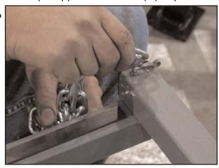
Insert Chain (I) into hook on side of Panel Rest (D). Repeat on other side of Panel Rest (D) with second Chain (I).
