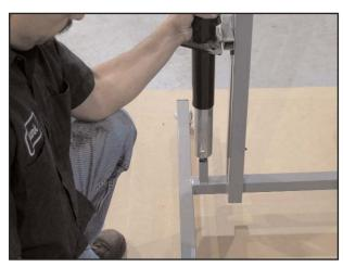
Place bottom of Panel Jack (B) onto post on the base of the Main Body (A).
