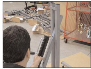
Slide top of Panel Jack (B) in between the two upper posts of Main Body (A).
