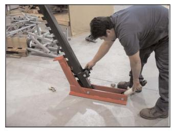
Remove bolt from ram coupler on post.c
