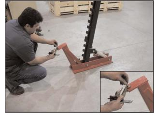
Attach hook to back of base by with supplied locking pin
