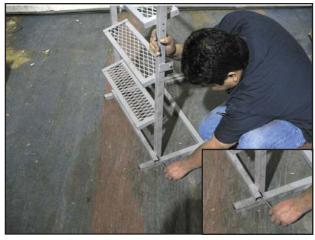
Insert the bolt on each side into the aligned holes and tighten the nut. Repeat for other side.
