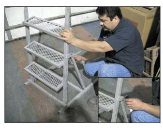
Remove the nuts and bolts on the side support. Adjust the side support so the holes aligne. Insert the bolt and tighten the nut on each side. Repeat for other side.
