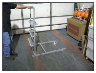
Unscrew the nut and remove the bolt from part A on each side. Line up the holes on part A and Part B. Keep Part B in an upright position.
