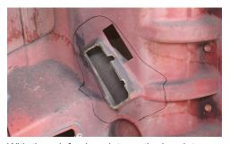
With the reinforcing plate on the hood, trace around it with a permanent marker to mark the area to be sanded.
