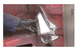
Place the reinforcing plate back on the hood and double check the fit. Make sure the plate can be fully seated over the entire surface and there are no large gaps at the edge of the plate where it meets the hood. PlastiFix is a very strong adhesive and will work well filling gaps up to about 1/8" wide, so perfection isn't needed. If there are large gaps, further trimming of the hood may be required to clear the aluminum reinforcing ribs.
