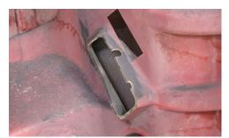
Removing the top of the bulge provides clearance for the reinforcing ribs on the repair plate to clear the hood, allowing the plate to be fully seated onto the hood's surface. The 1" (2.5 cm) wall provides extra bonding area between the plate and the hood.
