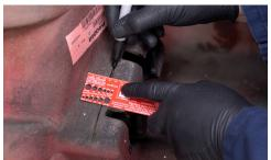
Measure approximately 1" up from the flat surface of the hood and draw a cut line all the way around the strut mount bulge.
