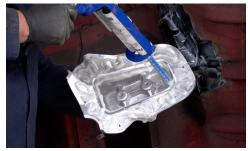
Apply an even larger amount of adhesive to the reinforcing plate, zig-zagging across entire sanded surface.
