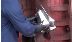
Test fit the plate to be sure it can be fully seated onto the hood. It should be snug, but if it does not seat with moderate pressure, trim a little more of the hood away until it can be fully seated.
