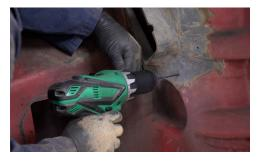
Once confirming the reinforcing plate can be fully seated, use the plate as a guide for marking the 6 locations for drilling 9/64" holes. The plate itself can be used as a drill guide, or drill at the marks as we have done here.
