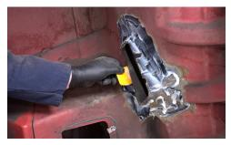
Apply a generous amount of adhesive to the surface of the sanded area on the hood. Use a body spreader to cover the entire area.
