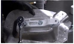
Before bonding the reinforcing plate to the hood, install the OEM bracket onto the reinforcing plate using the included 1-3/4" bolts, flat washer and lock washer, with the fork facing the large side of the bulge. A few drops of low strength thread locker on the bolts is recommended to reduce corrosion of the bolt in the threaded hole.
