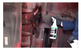
Clean the area to be repaired with soap and water, then 1000 Super Prep or 1001-4 EcoPrep to remove all contaminants from the surface. Gently force dry the area with a heat gun if necessary.
