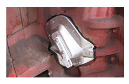
After curing a minimum of 4 hours at room temperature, or 24 hours for full strength, it's safe to attach the hood struts. Be sure the hood struts are functioning properly before mounting them, as this is typically the reason the mounts failed in the first place.
