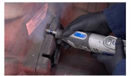
In a well-ventilated area, use a rotary tool with a cut off wheel to remove the top of the bulge.
