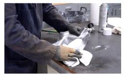
Blow the dust off the mating surfaces and clean a second time with 1000 Super Prep or 1001-4 EcoPrep. Wipe dry with a clean dry cloth. Make sure the surfaces are completely dry before proceeding to the next step.
