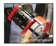
Keep your blades sharp! This is crucial for effective cutting action and tool longevity. A dull blade will destroy the drive mechanism in your Equalizer® tool. Sharpen the blade between each removal with a diamond file. Be careful to maintain the original sharpening angle.
