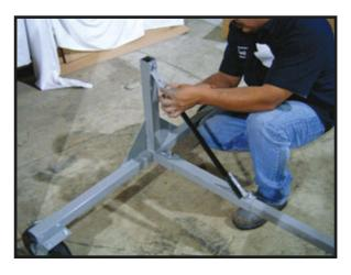
Attach Base Support Bracket to Vertical Base Support & Support Crossmember. Repeat for both sides.
