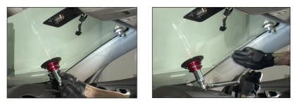
Continue cutting down the A-pillar until the wires cross making the final cut and the wire simply reels back into the vehicle. The removal is complete. You can now remove the mini anchor and Viper<sup>™</sup> unit and proceed to lift out the windshield and prep for replacement.
