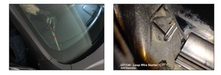
Note: To avoid damages to the painted area it is recommended to place a piece of tape on the exterior of the pinchweld.
