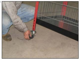
Carefully lift each corner of the unit and screw each Caster onto the bottom of each Corner Upright
