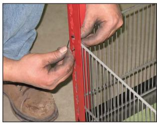
Feed Fencing Ties through the Fencing Piece and the Corner Upright and fasten it securely at the top and bottom of each piece.
