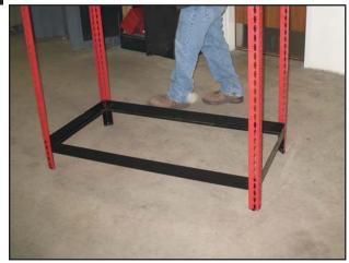
You should now have 2 long and 2 short cross beams inserted into all 4 corner uprights as shown above.
