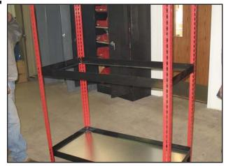
Work your way around all 4 sides on the Deluxe Parts Station inserting cross beams until you have all 4 sides done as above.
