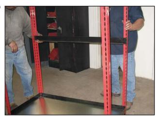
Insert Cross Beams into the Corner Uprights at the middle of the Corner Upright (or desired location) for the second shelf the same way you did for the bottom shelf.
