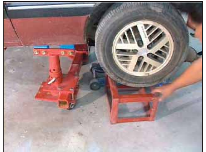
Raise vehicle to remove wheel stands and lower into Pinchweld Clamps
