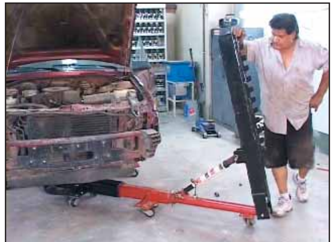
Each pulling tower has two swivels for extended reach. Remove locking pin, swivel into desired position and reinsert locking pin.
