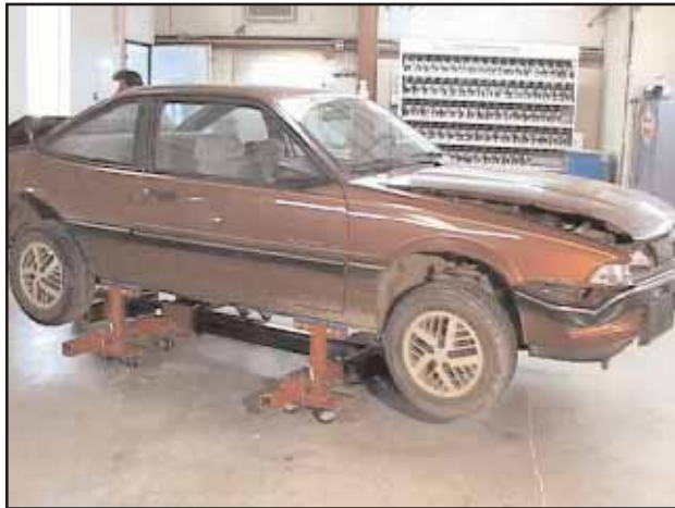
Vehicle is now attached to Xtreme and you are ready to attach Pulling Towers. Insert tower into desired tower insert and lock into place with locking pin.
