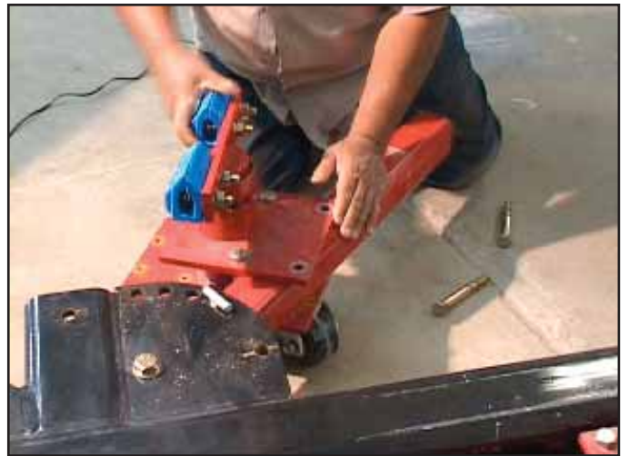
Remove Pinchweld Clamp Brackets.
