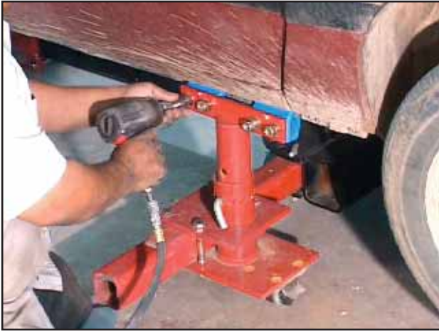
Tighten Pinchweld Clamps securely onto vehicle pinchwelds.
