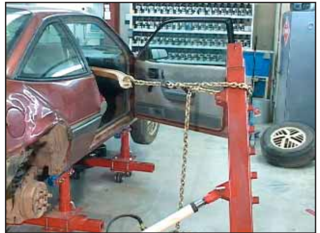
Wrap chain around Pulling Tower and lock into place using chain lock or pulling hook. Chain height is adjustable by positioning chain against the desired lock on tower.
