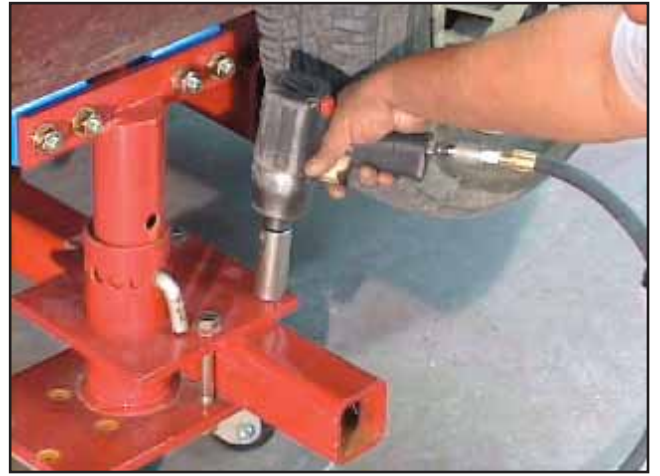
Tighten Pinchweld Brackets securely to Bracket Arms.
