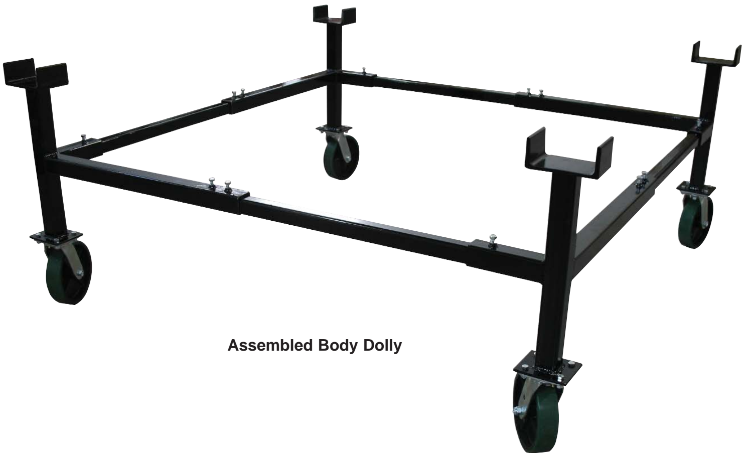
Adjust Dolly to desired width by sliding extension arms in or out and then securely tightening the locking bolts. For safety reasons NO RED PAINT should be showing on the Extension Arms. If red paint is visible then slide bracket into the the Corner support arm until it is no longer showing.
