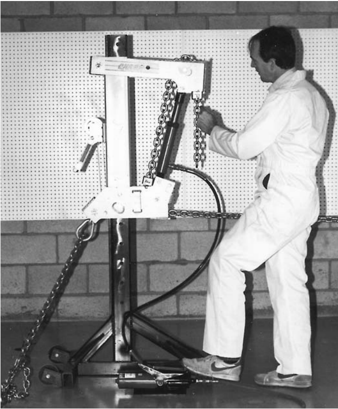
5. Holding top chain lock in place, continue raising ram until pressure holds it in place.
