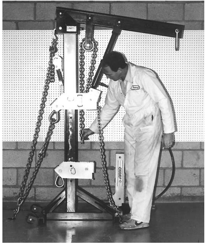
6. Lower chain through pulling mechanism toward double pull kit as shown. Two chains will be joined at this point.
