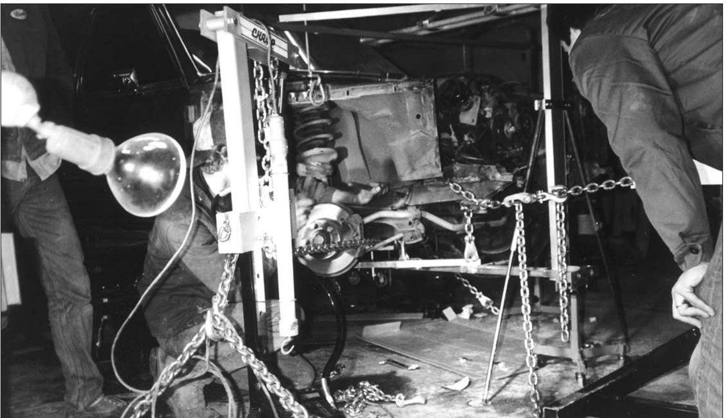
MULTIPLE PULL ON FRONT END. LITTLE CHAMP PULLS CROSSMEMBER BACK TO CENTER AND BIG CHAMP RESTORES LENGTH TO RIGHT RAIL. TECHNICIAN STRESS - RELIEVES BUCKLE IN RAIL WITH BOTH POSTS UNDER TENSION.
