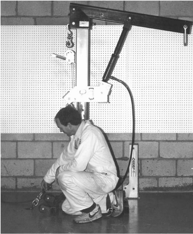
1. Position post in front of anchor and install claw sling on anchor chain.
