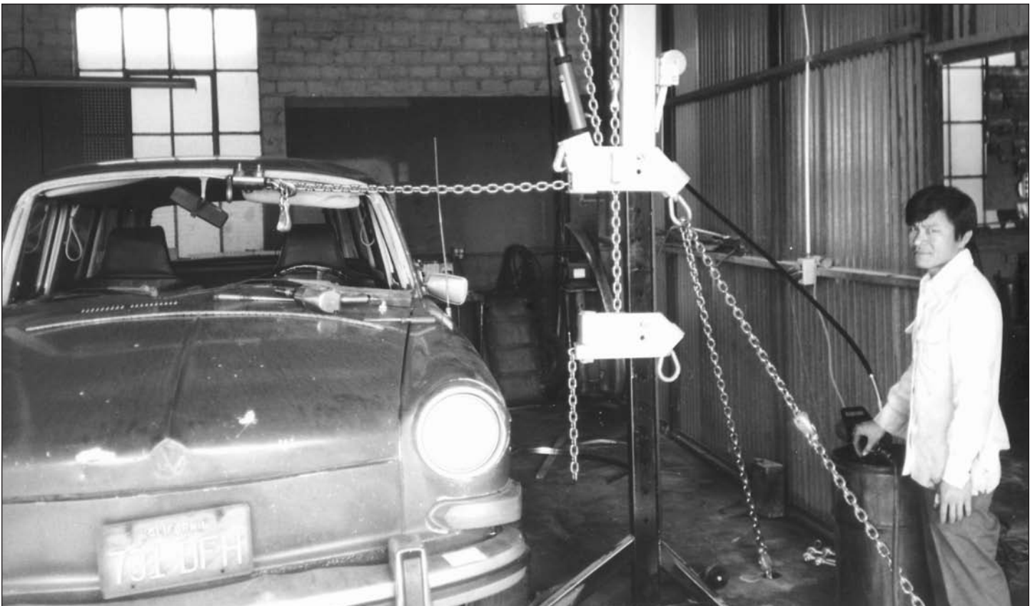
HOOKUP WITH CHAMP 3-WAY CLAMP. TECHNICIAN READY TO PULL.
