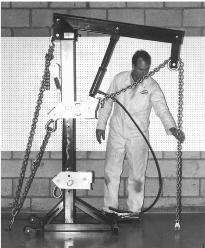
3. Using triple pull kit attachment in the fashion shown, attach chain to horizontal pin with double claw.
