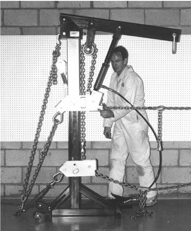
11. Install chain lock onto front on pulling mechanism to isolate lower pull.
