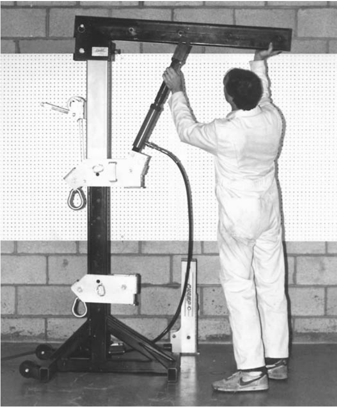
5. Position the pushbar over the middle hole of the beam.
