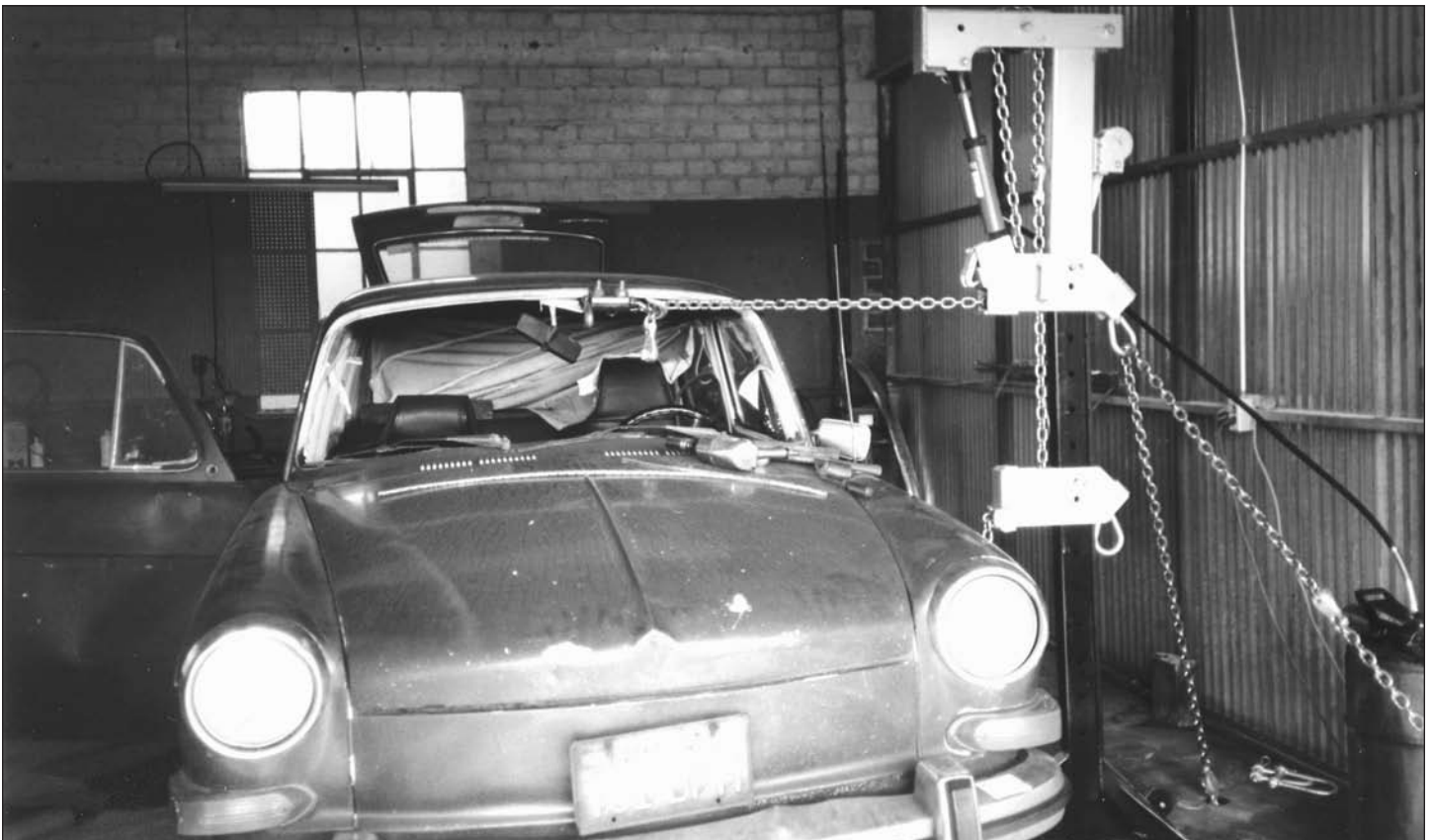
FINISHED PULL RESTORES WINDSHIELD OPENING.
