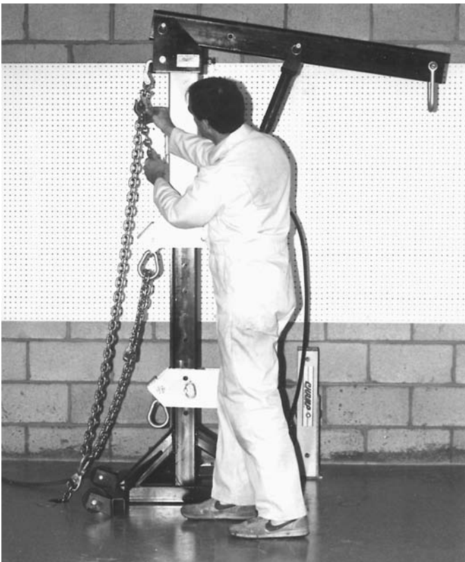
3. Install opposite end of chain onto hook on end of anchor claw at rear on hinge bracket.
