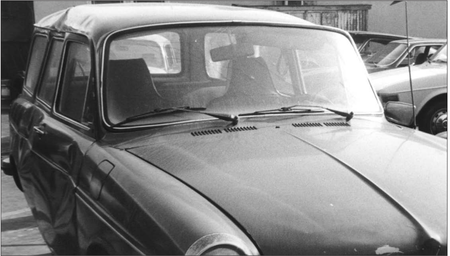
ROLLOVER COLLISION CAUSES WINDSHIELD OPENING TO BE SEVERLY DISTORTED.
