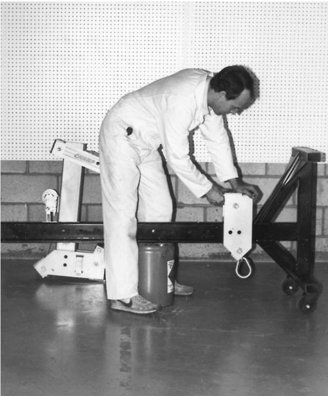
11. Continue sliding double pull kit all the way to the end of the post.
