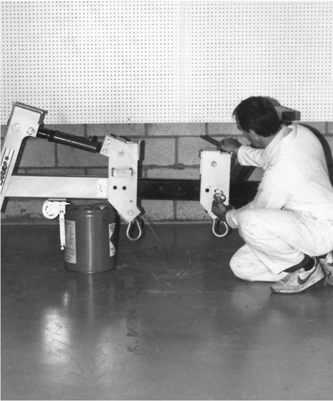
13. Insert height pin for double pull kit securing it to the post.
