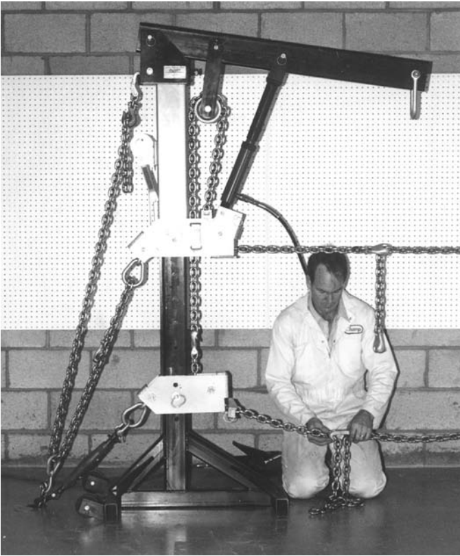
9. Attach second chain to damage.
