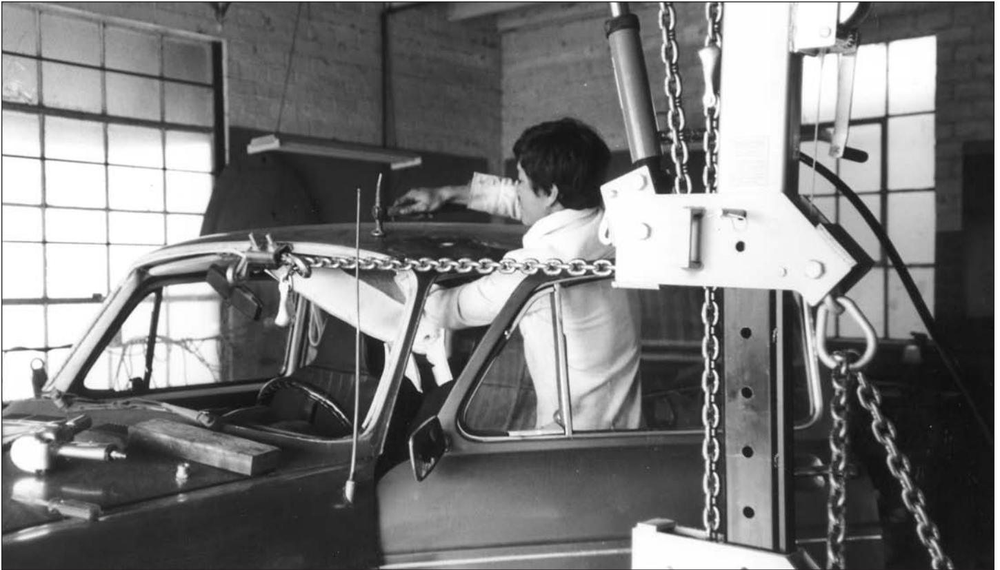
TECHNICIAN STRESS-RELIEVING DAMAGE UNDER TENSION.
