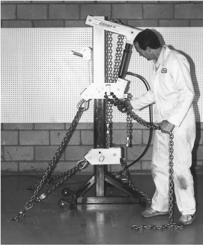
1. Thread chain through loop on side of pulling mechanism. Attach claw to chain.
