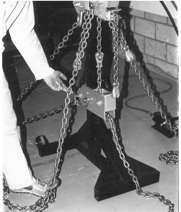
4. These chains remain slack during pull. In the event of breakaway, post will not fall over.
