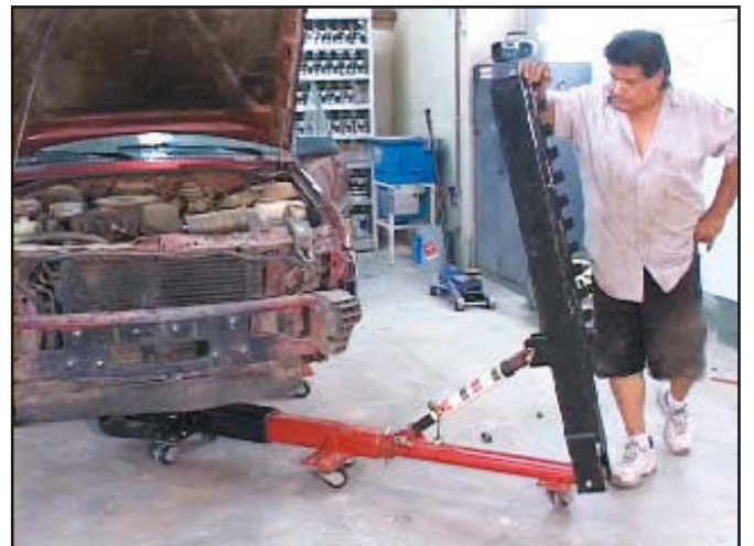
Each pulling tower has two swivels for extended reach. Remove locking pin, swivel into desired position and reinsert locking pin.
