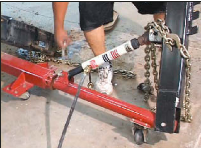
Each pulling tower has two swivels for extended reach. Remove locking pin, swivel into desired position and reinsert locking pin.
