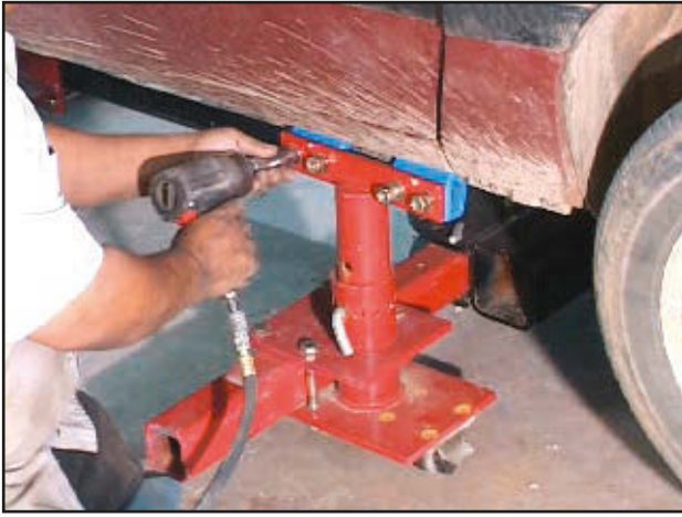
Tighten Pinchweld Clamps securely onto vehicle pinchwelds.
