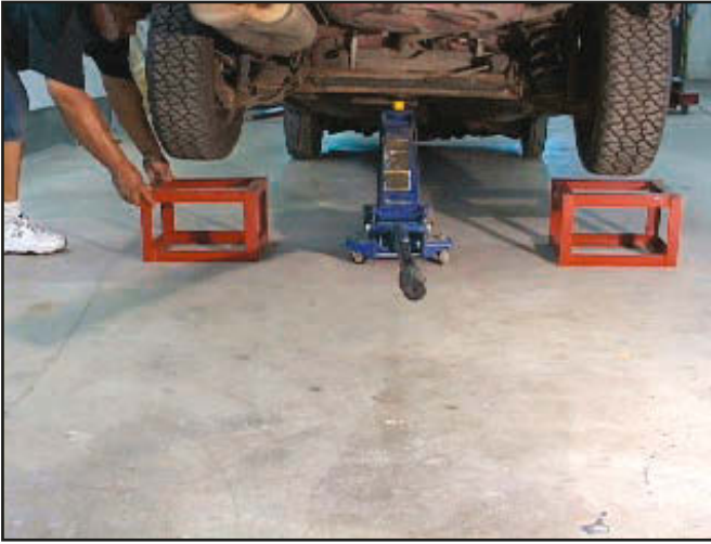
Raise vehicle and lower onto supplied vehicle stands.
