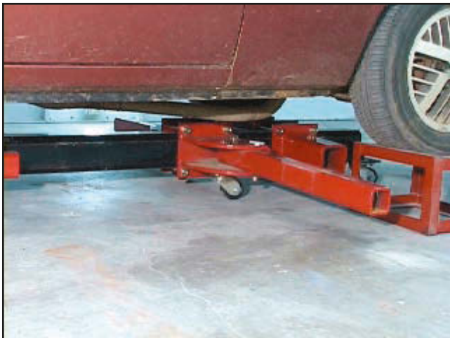
Swing Bracket arms back out. Reinstall Pinch weld Clamp Brackets & Pinch weld Clamps.
