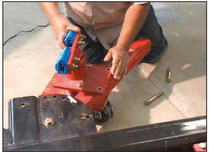
Remove Pinch weld Clamp Brackets.
