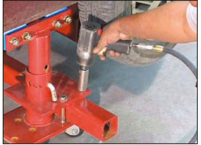
Tighten Pinchweld Brackets securely to Bracket Arms.
