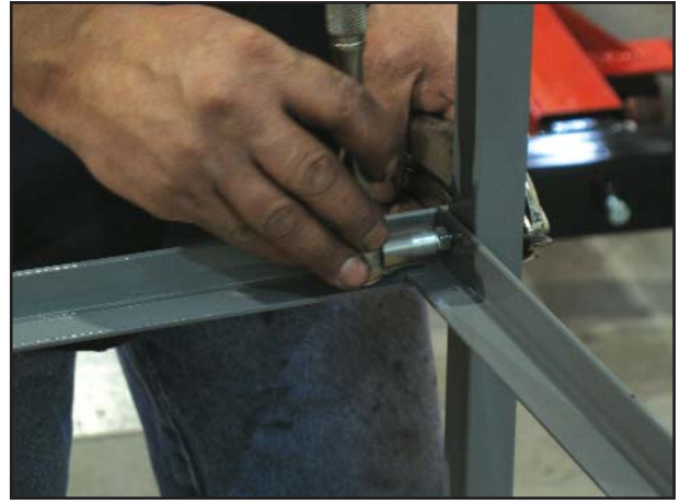
Select your desired final angle of parts rack and fully tighten all bolts.
