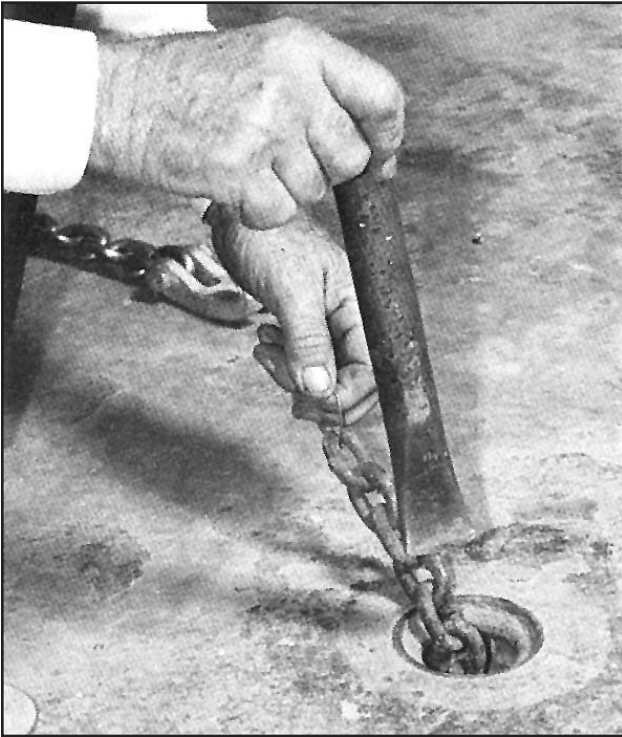
1. Pull chain aside to make room for blunt instrument to be used as a driver.
