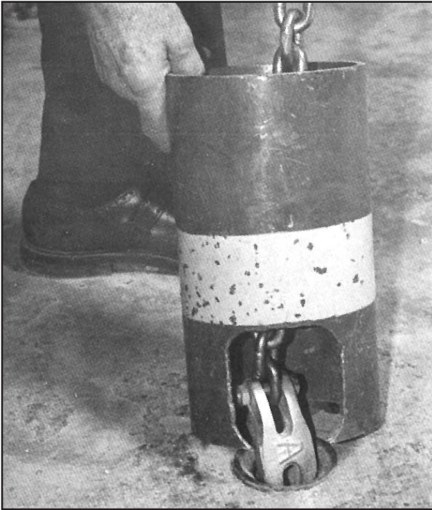
5. Position remover tube over anchor as shown with puller claw and chain.
