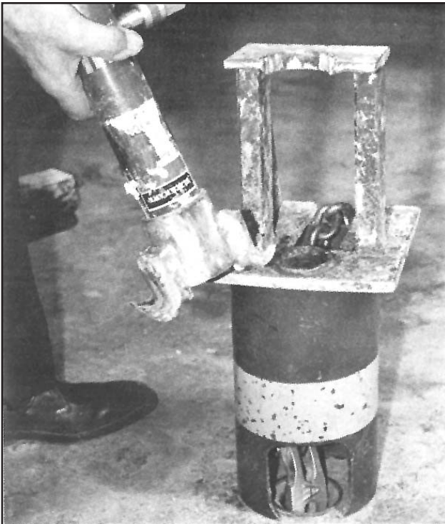
7. Install ram and puller claw assembly into press if not already prepared.
