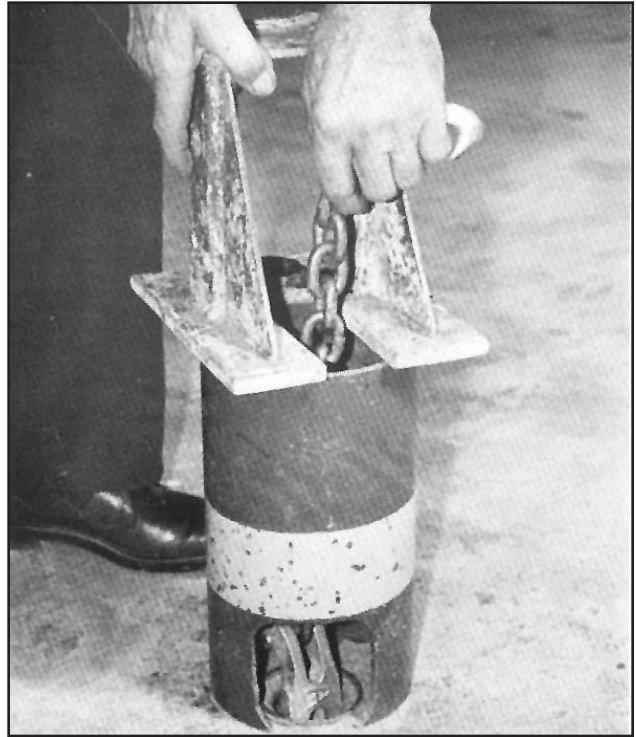
6. Position anchor press over puller tube as shown with chain protruding from opening.
