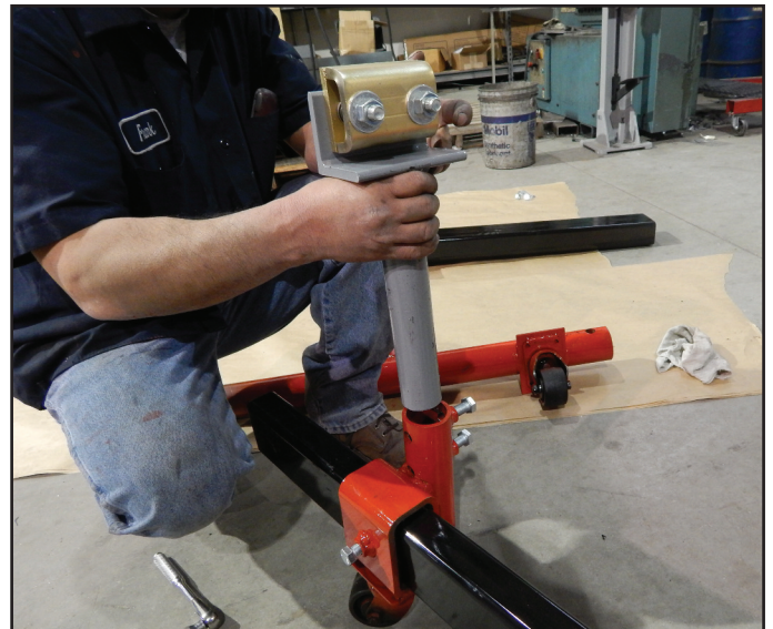
16. Attach the Pinchweld Clamp Assembly (G) to the Pinchweld Clamp Mounting Base (F).
