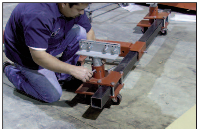
Clamps are adjustable for Front & Side Pulls
