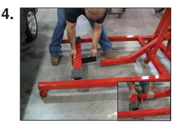
Slide the assembled adapter into the lift beam of the lift. Lock it into place with the supplied locking pin.
