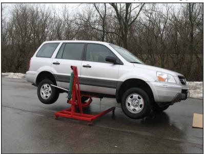
Your lift is now ready to use. Make sure that the lift pads are placed in an approved lifting section of the car. Contact the vehicle manufacturer if you are not sure where to place the lifting pads.
