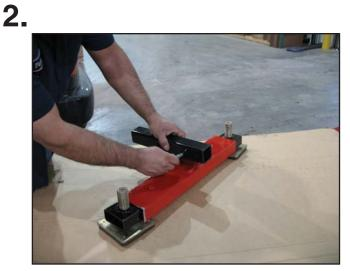
The adapter attaches to the cross beam adapter with the supplied bolt.
