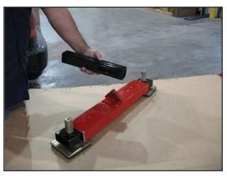
The jack beam adapter has a slot one side.
