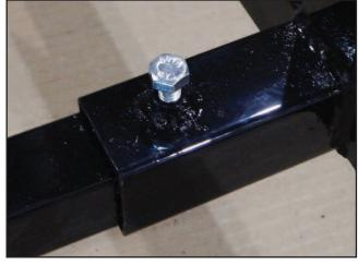
Secure the bottom support beams (C) to the wheel bases (A) with supplied bolts.
