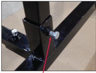
Secure the 46" uprights (E) to the wheel base (A) using supplied bolts (L). Do this to both sides.
