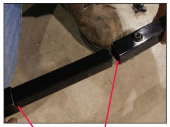
Slide the 12" bottom support connector (D) into each end of the bottom support beams (C)
