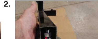
Secure the wheels (B) with supplied washers and nuts
