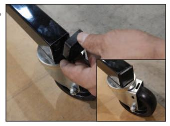
Install end caps (J) on the ends of the wheel bases (A).
