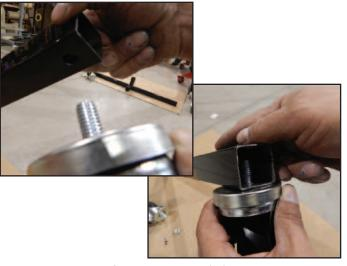
Insert the bolt of each wheel (B) into the bottom of both wheel bases (A)
