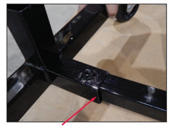
Slide the 41" bottom support beam (C) into the wheel base (A), as far as it will go. Both bottom support beams have welded nuts on them. Make sure these welded nuts are facing up. Repeat this step with the other side.
