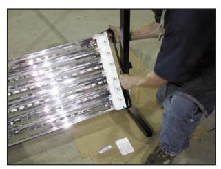
Place protruding 2" bolt (D) through provided hole in the bottom of upright Frame Structure (A). Place Hand Knob (E) on outside of Frame Structure (A) and tighten. Repeat on both sides.
