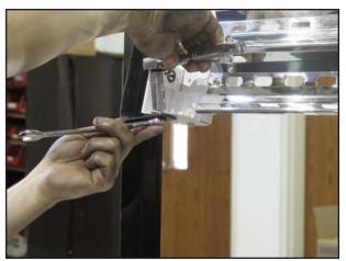
Fully tighten all nuts on brackets (included and already pre-assembled) on Light Housings (C).
