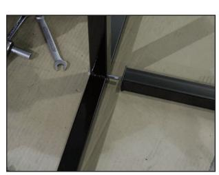
Attach straight bar of the Frame Structure (A) with 3" bolt (B)
