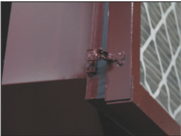
Close hinged door an lock into place with clasps at both sides.
