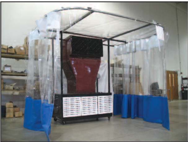
Hang curtains onto the curtain rail by inserting the roller hooks through the mounting holes on curtain.
