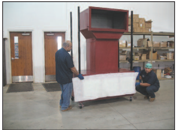
Install one prefilter across the front of the filters.
