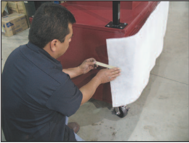
Mount prefilters by taping to the sided of the paint station.
