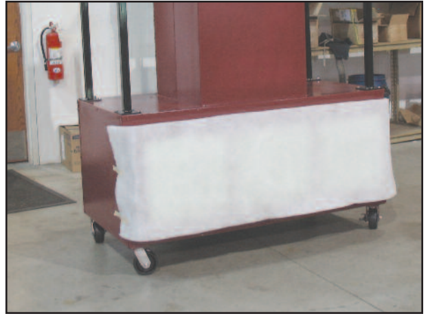
Inexpensive prefilters are used to prevent tri-fold filter from having to be replaced often. Simply replace prefilter as it gets dirty.
