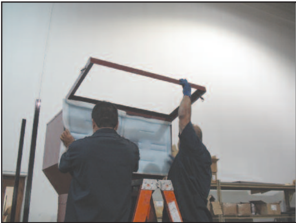
Install top filters. Open hinged door and install two exhaust panel filters with tacky side facing in.
