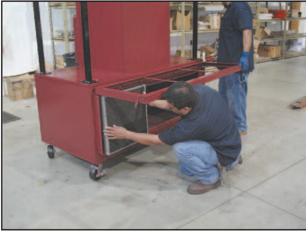
Lift hinged filter door and insert three metal framed carbon filters.
